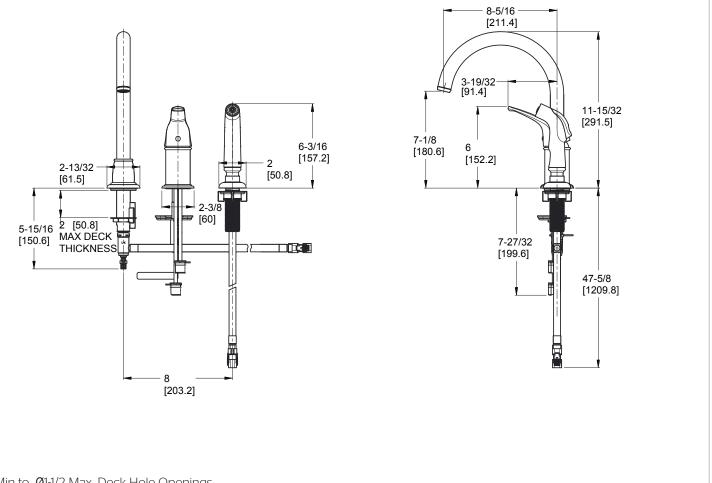
Ø1-3/8 Min to Ø1-1/2 Max. Deck Hole Openings
